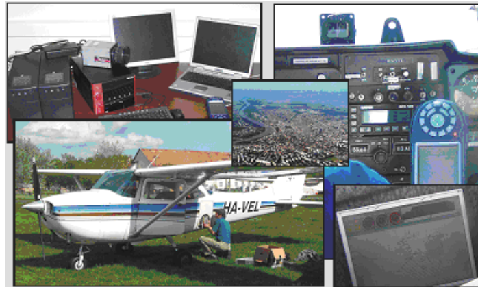
Figure 1. The different components of the data acquisition system (from top left to bottom right): computer and camera, the cockpit and the navigational GPS, the airplane, an overview photo over the city, navigation laptop
